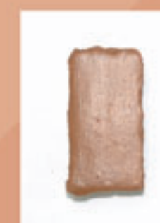
Briquette experimentally fired for 10 hours at 950^\circ\text{C}
