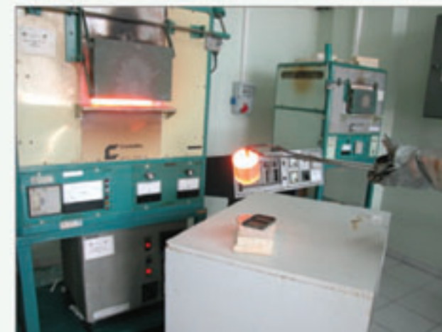
Frit making in the laboratory
